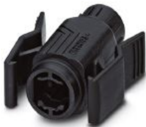
RJ45 sleeve housings, degree of protection: IP67, number of positions: 8, material: PA, cable outlet: straight, color: jet black RAL 9005
