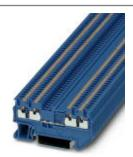
Feed-through terminal block, nom. voltage: 500 V, nominal current: 17.5 A, connection method: Push-in connection, number of connections: 4, cross section: 0.14 mm² - 1.5 mm², AWG: 26 - 14, width: 3.5 mm, height: 30.5 mm, color: blue, mounting type: NS 35/7,5, NS 35/15
