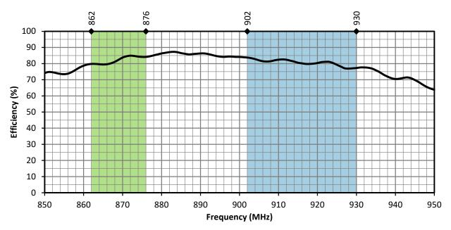
Figure 8. Antenna Radiation Efficiency for ANT-8/9-PW-LPN, Edge of ground Plane
