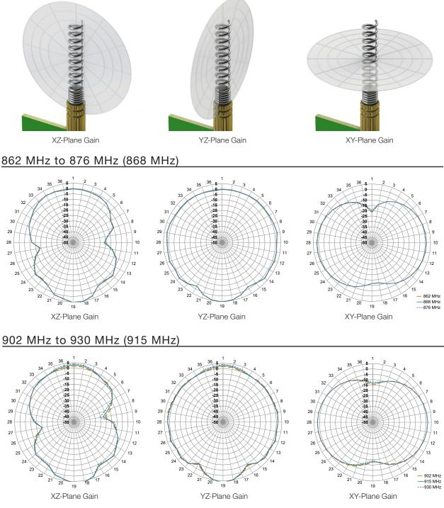
Figure 9. Radiation Patterns for ANT-8/9-PW-LPN Antenna, Edge of ground Plane
