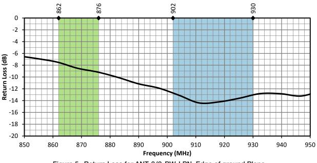
Figure 5. Return Loss for ANT-8/9-PW-LPN, Edge of ground Plane
