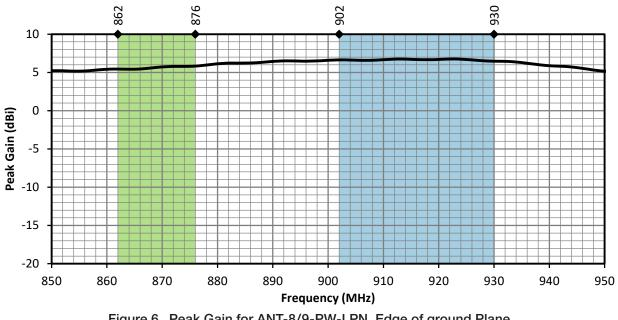
Figure 6. Peak Gain for ANT-8/9-PW-LPN, Edge of ground Plane
