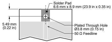
Figure 2. ANT-8/9-PW-LPN Recommended Mounting and PCB Footprint
