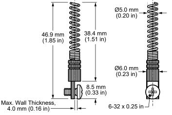
Figure 1. ANT-8/9-PW-LPN Antenna Dimensions
