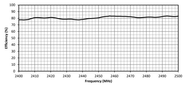
Figure 8. Antenna Radiation Efficiency for ANT-2.4-PW-LPN, Edge of ground Plane
