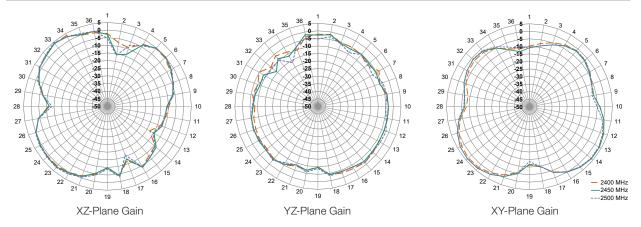
Figure 9. Radiation Patterns for ANT-2.4-PW-LPN Antenna, Edge of ground Plane
