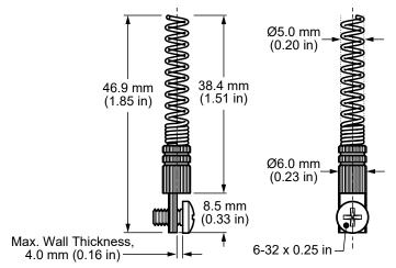
Figure 1. ANT-2.4-PW-LPN Antenna Dimensions
