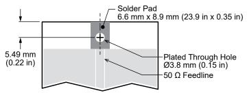
Figure 2. ANT-2.4-PW-LPN Antenna Recommended Mounting and PCB Footprint
