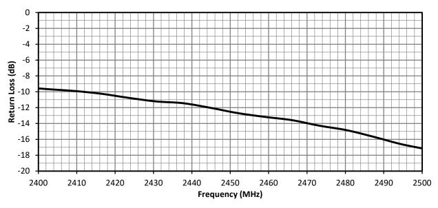
Figure 5. Return Loss for ANT-2.4-PW-LPN, Edge of ground Plane
