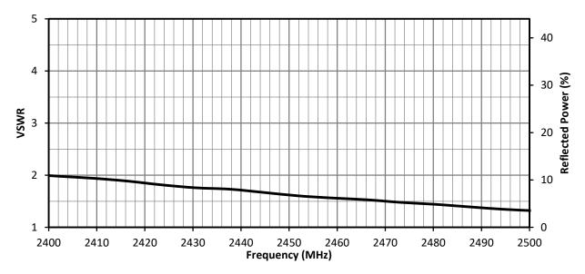
Figure 4. VSWR for ANT-2.4-PW-LPN, Edge of ground Plane
