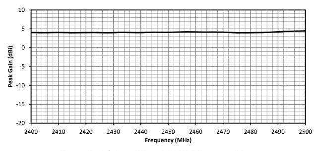
Figure 6. Peak Gain for ANT-2.4-PW-LPN, Edge of ground Plane
