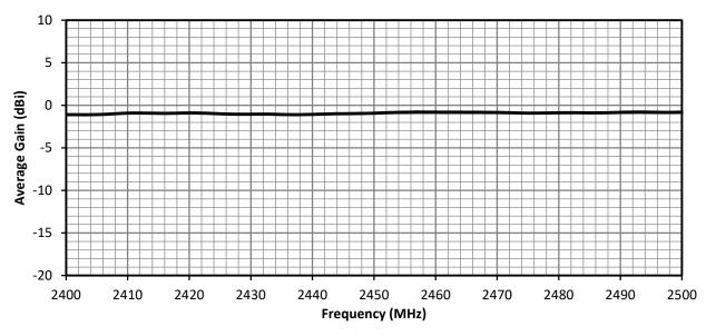
Figure 7. Antenna Average Gain for ANT-2.4-PW-LPN, Edge of ground Plane
