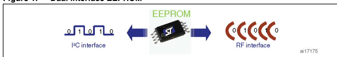
Figure 1. Dual interface EEPROM
