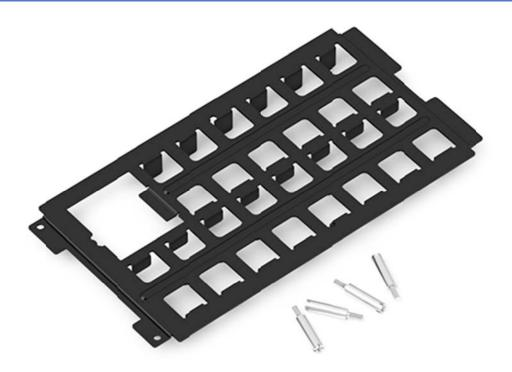
The vibration protection kit (VPK) consists of the vibration protection plate, four special screws, and two small rubber parts that cushion the <u>GA1000</u> Wi-Fi add-on, when installed (they come attached to the plate and are not visible on the above picture).
