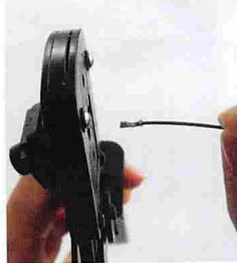
Remove the crimped contact.
