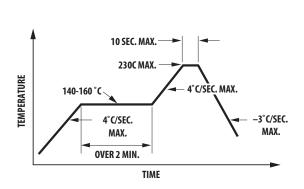
Figure 6. Recommended reflow soldering profile.
