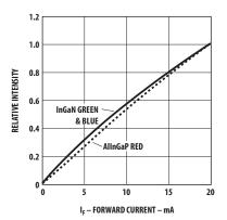
Figure 3. Luminous intensity vs. forward current.
