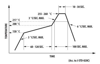
Figure 7. Recommended Pb-free reflow soldering profile.
