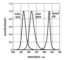
Figure 1. Relative intensity vs. wavelength.
