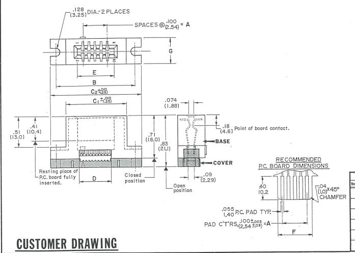
DIMENSIONS IN INCHES (METRIC-MILLIMETERS)
