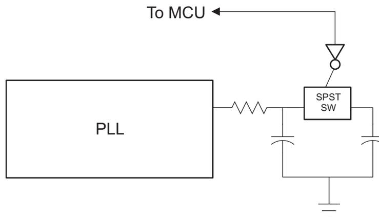
**Figure 22. Improved Lock Time Circuit Simplified Block Diagram**
