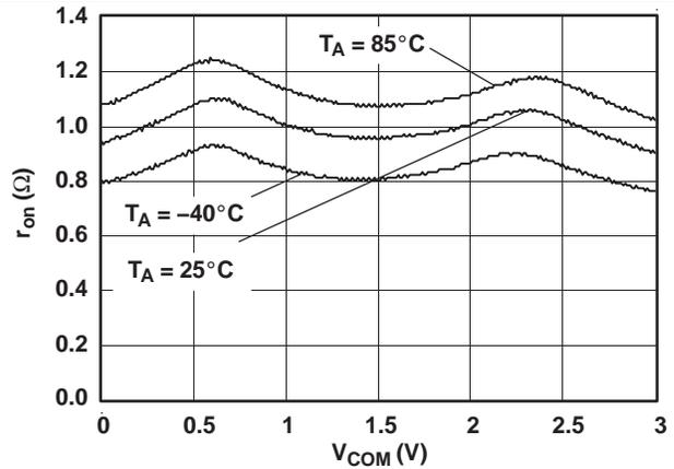
Figure 2.  $r_{on}$  vs  $V_{COM}$  ( $V_+ = 3V$ )
