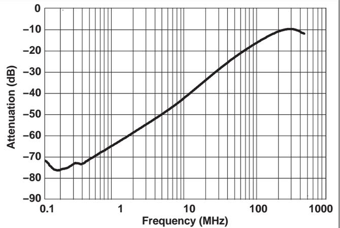
Figure 10. OFF Isolation vs Frequency ( $V_+ = 5\text{ V}$ )
