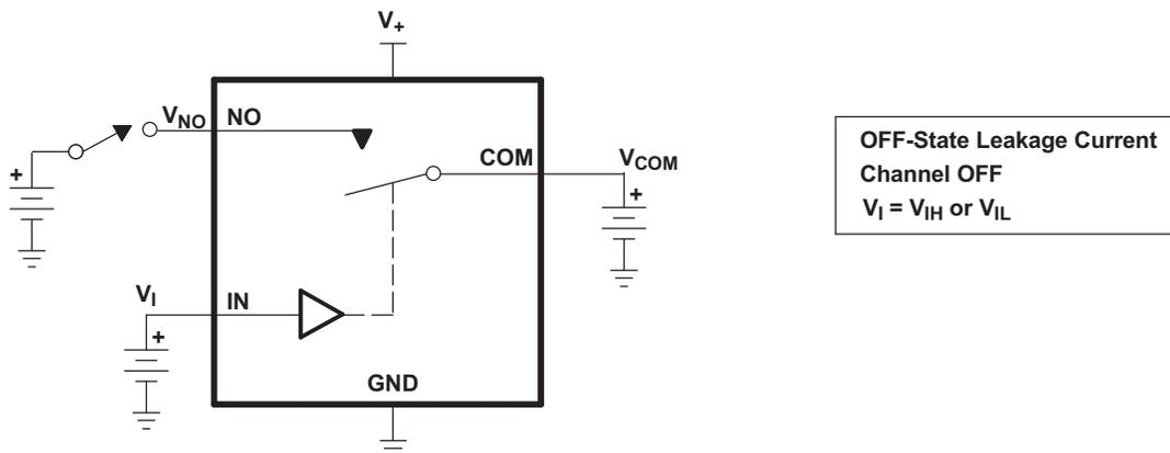
Figure 14. OFF-State Leakage Current ( $I_{COM(OFF)}$ ,  $I_{NO(OFF)}$ ,  $I_{COM(PWROFF)}$ ,  $I_{NO(PWRFF)}$ )
