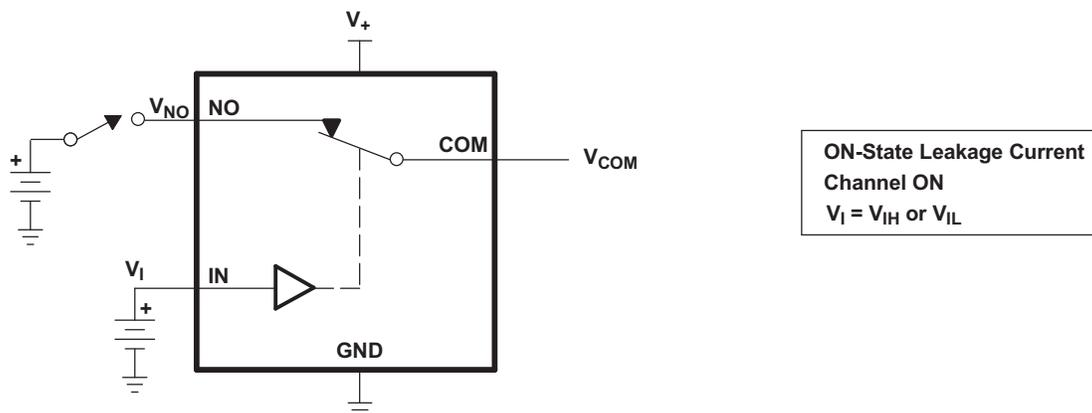
Figure 15. ON-State Leakage Current ( $I_{COM(ON)}$ ,  $I_{NO(ON)}$ )
