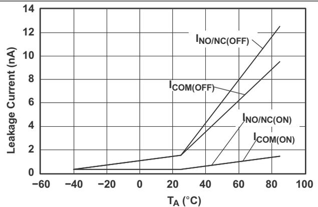
Figure 4. Leakage Current vs Temperature ( $V_+ = 5.5V$ )
