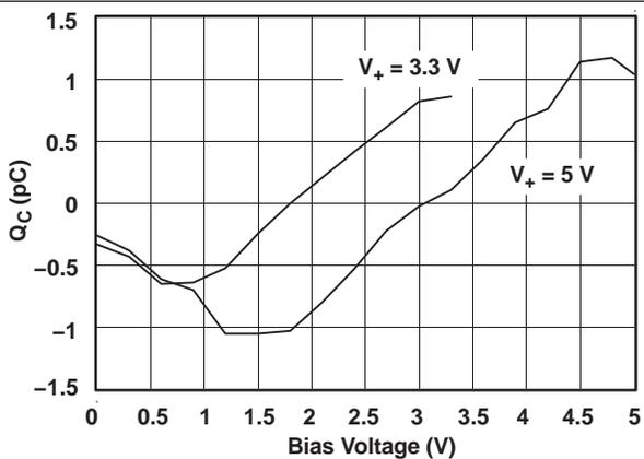
Figure 5. Charge Injection ( $Q_C$ ) vs  $V_{COM}$
