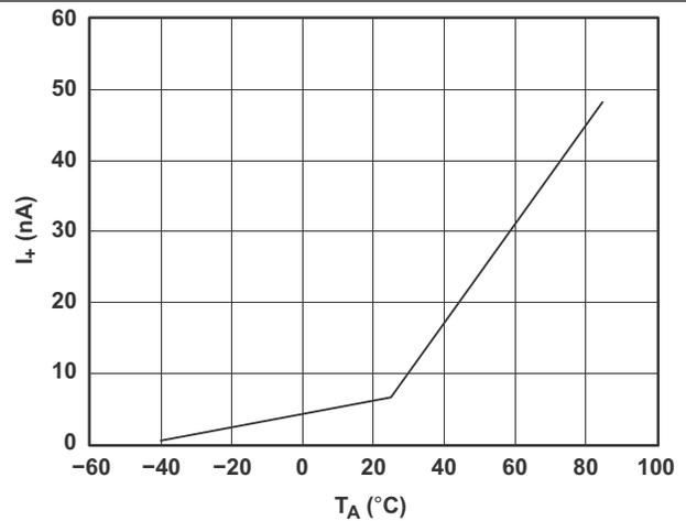
Figure 12. Power-Supply Current vs Temperature ( $V_+ = 5\text{ V}$ )
