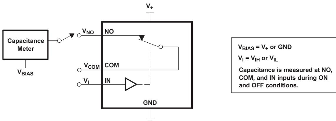
Figure 16. Capacitance ( $C_I$ ,  $C_{COM(OFF)}$ ,  $C_{COM(ON)}$ ,  $C_{NO(OFF)}$ ,  $C_{NO(ON)}$ )
