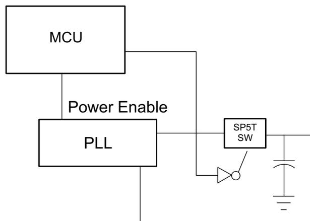
**Figure 23. PLL Improved Power Consumption Simplified Block Diagram**
