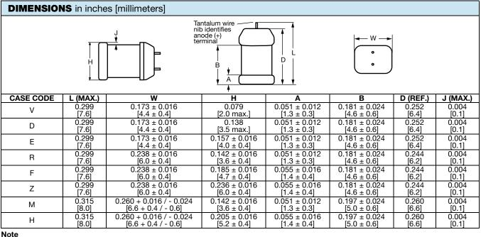
The anode termination (D less B) will be a minimum of 0.012" [0.3 mm]
