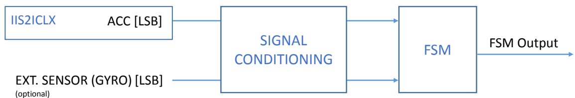
Figure 2. State machine in the IIS2ICLX
