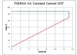
The idealized Constant Current characteristic is shown in the curves opposite. This feature will enable the PQU650 to successfully start in to application loads exhibiting large inrush current i.e. large capacitive loads, incandescent lamps, motors and solenoids. The curves are generated for the PQU650 variants by subjecting the output to an incremental (constant resistance) load, equivalent to 1Adc increments (above full load).
