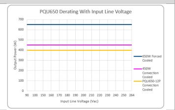
No derating with input line voltage for convection or forced cooling airflows for all variants in the series, except for PQU650-12P that derates to 400W when convection cooled.
