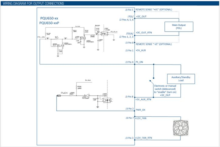
Note: For parallel (current share) operation it is required to connect the sharing power supplies in parallel (+DC out connected together and DC out Return connected together). Since each output has an identical "droop" share characteristic then each output will intrinsically share the total load current. See ACAN-107 for more details. It is recommended that for redundant (critical) applications that external isolation devices (diodes or MOSFETS) are employed; see ACAN-105 for suggested devices.
