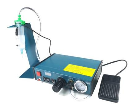
The SP1A Dispenser is used for precise control of pneumatically controlled dispensing of Liquids, Glues, Solderpaste etc. The material pressure can be precisely adjusted with the integrated compressed air regulator and allows for precision dispensing of Solderpaste and or adhesives etc. The unit has an adjustable time and vacuum suck back feature to aid accurate and easy dispensing.
