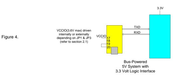
Figure 4 shows how to configure the DLP-2232H to interface with a 3.3V logic device via the ASYNC serial mode. In this example, the target electronics provide the 3.3 volts to power the microcontroller.
