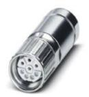
Cable connector, straight long, Screw locking, M23, number of positions: 5+PE, type of contact: Socket, shielded: yes, cable diameter range: 7.5 mm ... 18 mm, number of positions: 6, connection method: Crimp connection
