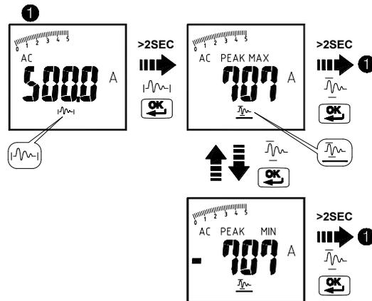
In PEAK HOLD mode, the meter is activated to save the positive peak value and negative peak value. Positive peak value is displayed in PEAK MAX mode. Negative peak value is displayed in PEAK MIN mode.
