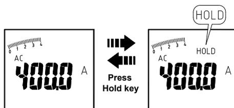
**SMART HOLD** : The meter will beep continuously and the display will flash if the measured signal is larger than the display reading. (for V, A, W, and Flex AC current function)
