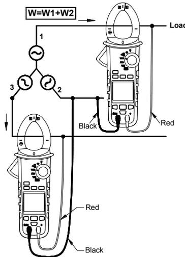
**b. 3-phase 4 wire balanced / unbalanced**
