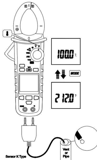
Don't take any high voltage measurement prior to accurate °C/°F measurements.
