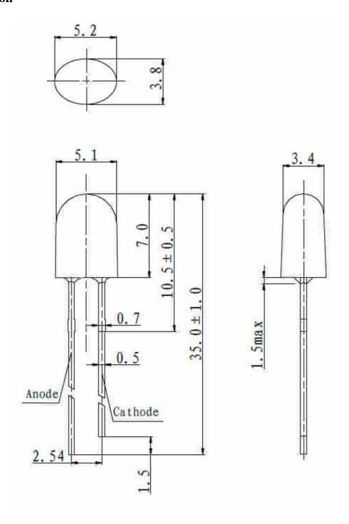
All dimensions in mm, tolerances unless mentioned is  $\pm 0.2$  mm.
