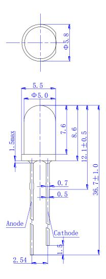
All dimensions in mm, tolerances unless mentioned is  $\pm 0.2$  mm.
