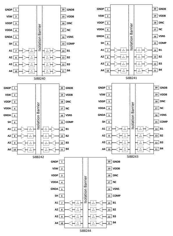
Figure 26. Si8824x Pin Configurations
