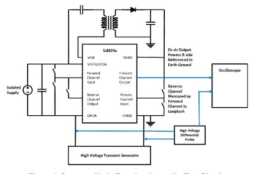
Figure 4. Common-Mode Transient Immunity Test Circuit
