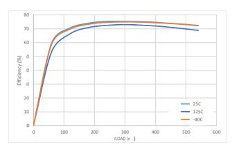
Figure 22c. Efficiency vs. Load Current over Temperature, 5.0 V-3.3 V
