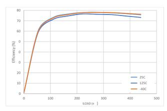
Figure 22d. Efficiency vs. Load Current over Temperature, 5.0 V-5.0 V
