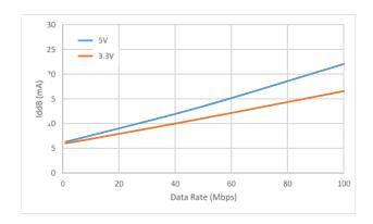
Figure 17. Si88241 Typical V<sub>DDB</sub> Supply Current vs. Data Rate 5 and 3.3 V Operation
