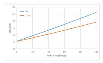
Figure 13. Si88242 Typical V<sub>DDA</sub> Supply Current vs. Data Rate 5 and 3.3 V Operation
