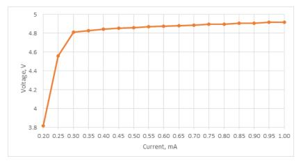
Figure 25. Typical I-V Curve for VREGA/B
