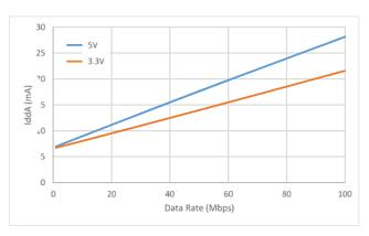
Figure 12. Si88241 Typical V<sub>DDA</sub> Supply Current vs. Data Rate 5 and 3.3 V Operation
