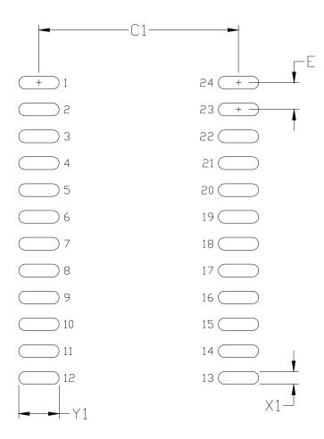
Figure 33. 24-Pin SOIC PCB Land Pattern
