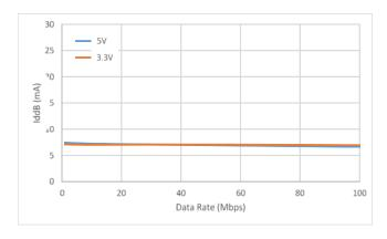
Figure 18. Si88242 Typical V<sub>DDB</sub> Supply Current vs. Data Rate 5 and 3.3 V Operation
