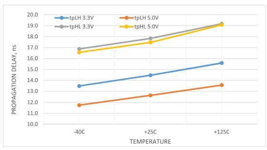
Figure 21. Propagation Delay vs. Temperature
