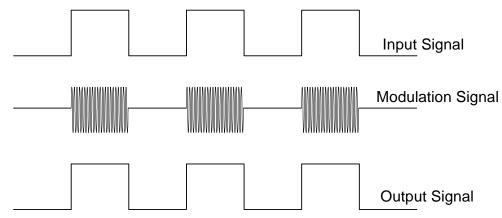
Figure 7. Modulation Scheme
