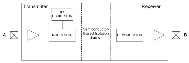
Figure 6. Simplified Si88xx Channel Diagram
