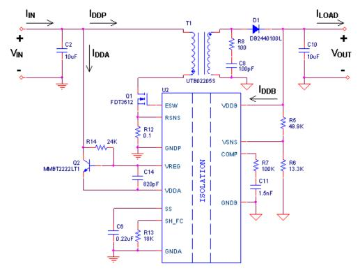
Figure 3. Measurement Circuit for Converter Efficiency and Regulation for Si884xx, Si886xx
