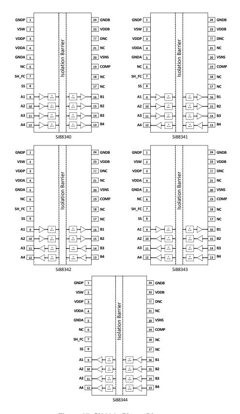
Figure 27. Si8834x Pinout Diagrams
