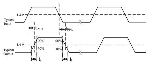
Figure 1. Propagation Delay Timing for Digital Channels
