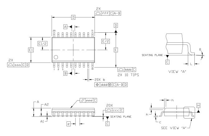
Figure 30. 20-Pin Wide Body SOIC
