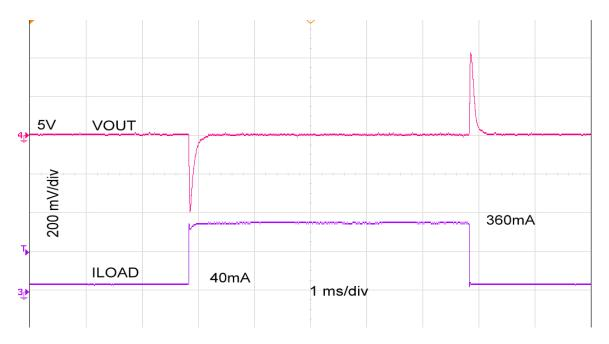
Figure 24. 5 V-5 V VOUT Load Transient Response, 10% to 90% Load
