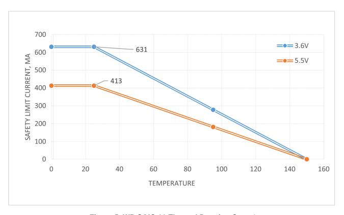
Figure 5. WB SOIC-20 Thermal Derating Curve\*
