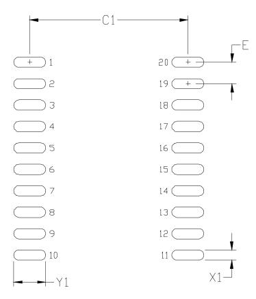
Figure 31. 20-Pin SOIC PCB Land Pattern
