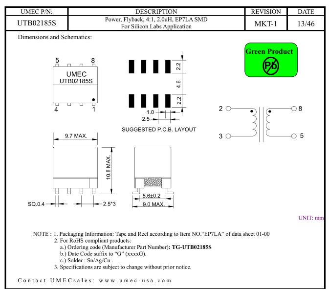
**Figure 10. Transformer Specification**
