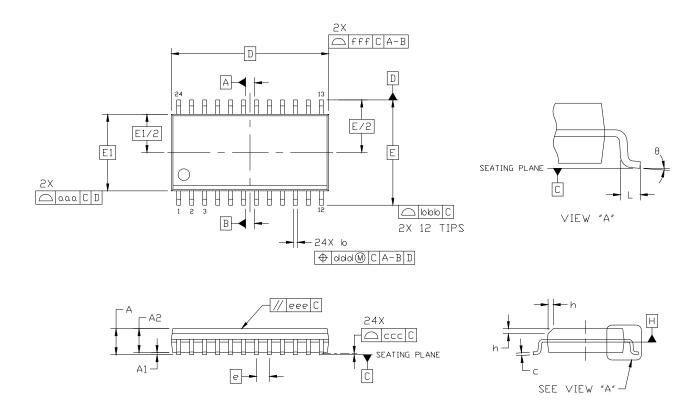
Figure 32. 24-Pin Wide Body SOIC
