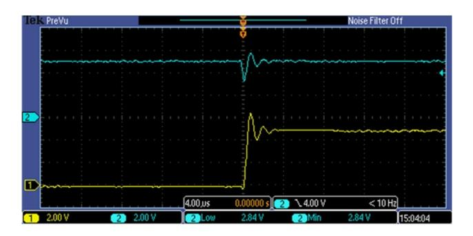
This time the power-on only causes a pulse in small magnitude. No reset turns up because the pulse only lasts about 1us.
