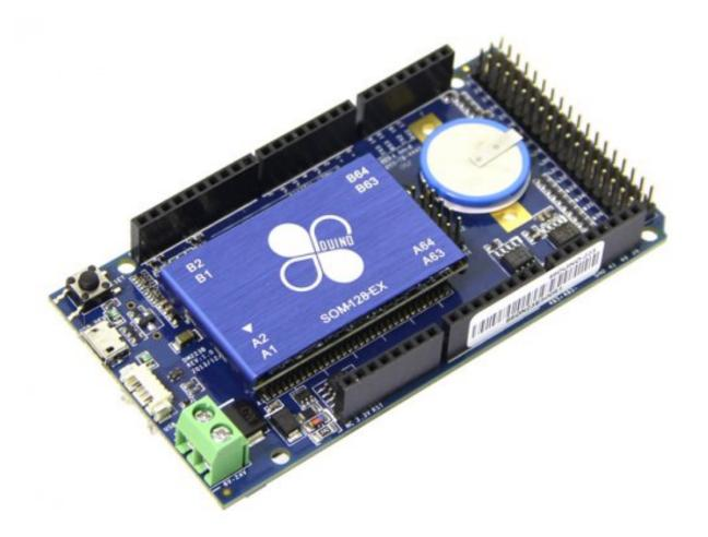
86Duino is an open-source embedded platform based on Vortex86EX SoC, easy-to-use hardware and software integrated. This Arduino-compatible board can support many x86 O/S as well as those running on the original Arduino base system.
