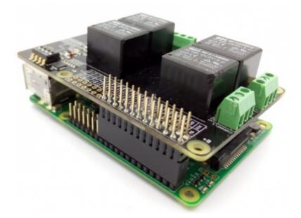
The Relay Shield utilizes four high quality relays and provides NO/NC interfaces that control the load of high current. Which means it could be a nice solution for controlling devices that couldn't be directly controlled by IIC bus. Standardized shield form factor enables smoothly connection with the Raspberry Pi . The shield also has four dynamic indicators show the on/off state of each relay.
