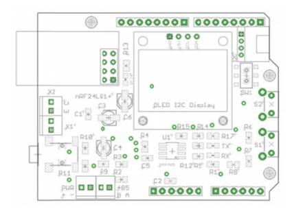
The left side of EM Shield is a connector for current sensors (terminals X1 and X1 '- duplicate each other).
