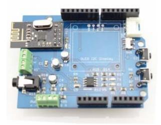
Energy Monitor Shield v2 is an Arduino-compatible expansion card designed for building energy monitoring system with support I2C OLED display, with the phototransistor to read data from the built-in LED for different energy meters, interface RS485 and built-in wireless transceiver nRF24L01 +.
