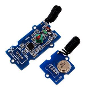
This kit is used for one way wireless communication at a frequency of 433MHz and includes a transmitter module and a receiver module. The twig configuration of this kit allows for around 40 meters of transmitting distance indoors, or around 100 meters outside.
