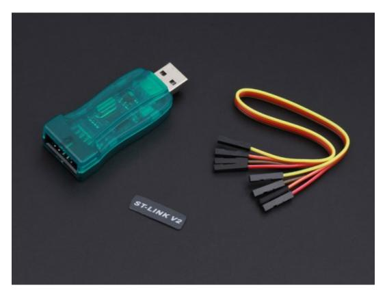
The ST-LINK/V2 is an in-circuit debugger and programmer for the STM8 and STM32 microcontroller families. The single wire interface module (SWIM) and JTAG/serial wire debugging (SWD) interfaces are used to communicate with any STM8 or STM32 microcontroller located on an application board.
