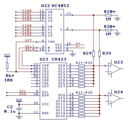
The OC pin of CH423 in the open-drain output mode is a low-resistance open-drain output pin, has the on resistance less than  $10 \Omega$ , and can be used as an analog switch with one end grounded. After multiple OC pins are connected with their respective external resistors and combined for turn-on, a digital programmable resistor with one end grounded can be formed.
