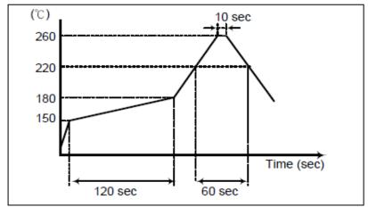
The reflow temperature profile may vary depending on the product model, specifications and frequency range.Refer to the individual product specifications for details
