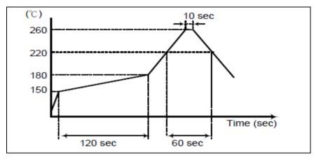
The reflow temperature profile may vary depending on the product model, specifications and frequency range.Refer to the individual product specifications for details
