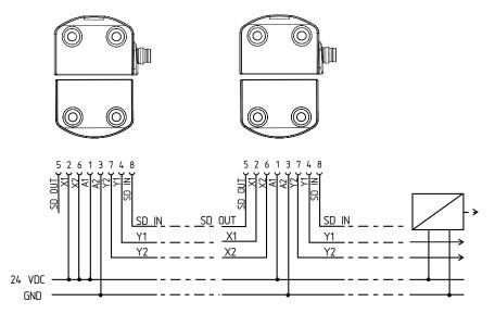
Y1 and Y2 = Safety outputs  $\rightarrow$  dual-channel safety monitoring module SD-IN  $\rightarrow$  Gateway  $\rightarrow$  Field bus
