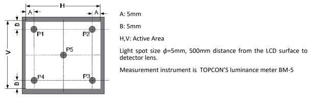
Figure 3. The definition of viewing angle
