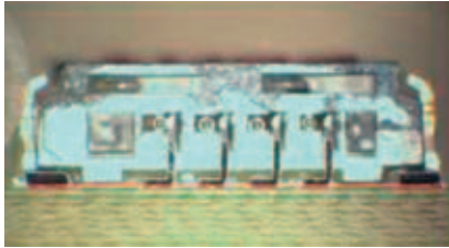
Cross Section Right Angle Male Connector
