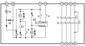
Note: 1. For 1-channel input with G9SB-□□□-B/D models, short terminals T12 and T22. It is not possible to wire G9SB-□□□2-A/C models for 1-channel input.
