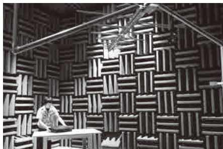
Acoustic radio wave anechoic chamber
