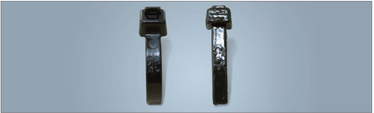
GalvaLok and PA66 ties after 24 hours in a saturated zinc chloride solution at +90°C.
