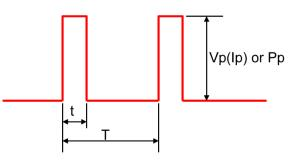
Where: Vp: Pulse limiting voltage (V)
