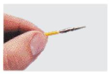
**1** Grasp contact approximately (25.4 mm) one inch behind the contact crimp barrel.
