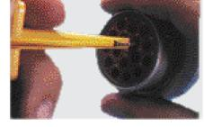
**3** Pull contact-wire assembly out of connector.
