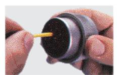
**3** Push contact straight into connector grommet until a positive stop is felt. A slight tug will confirm that it is properly locked in place.
