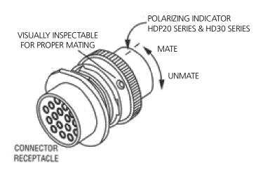
CAUTION: When mating or unmating plug and receptacle, disassemble by hand. DO NOT use pliers or any other tool.
