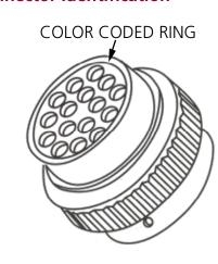
Color code is visible from the rear of the receptacle or plug.
