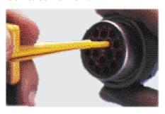
**1** With rear insert toward you, snap appropriate size extractor tool over the wire of contact to be removed.
