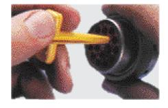
**2** Slide tool along into the insert cavity until it engages contact and resistance is felt.
