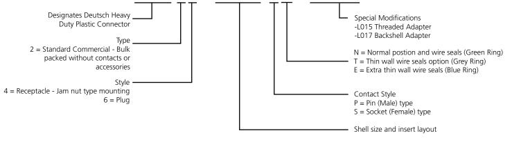
Deutsch HD30 Series contacts, sealing plugs and tooling are specified for use in the HDP20 Series. Consult factory for additional options and special modifications available.
