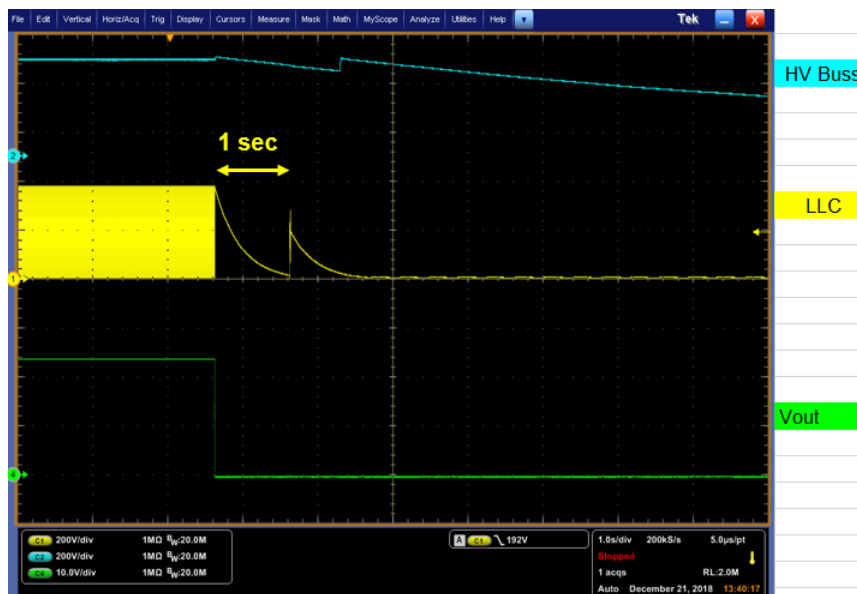
Figure 26 – Permanent short occurring
