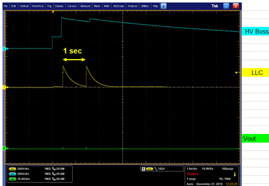
Figure 24 – Power-up into a shorted output
