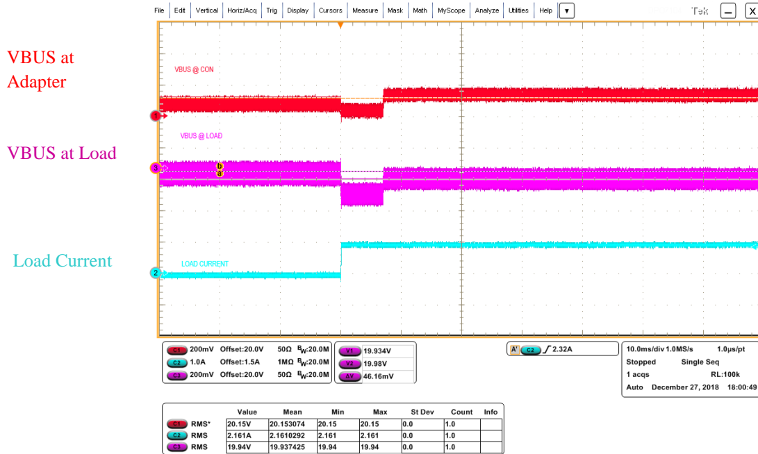
Figure 4 – 1.5A to 2A load step to induce 100mV/A VBUS increase
