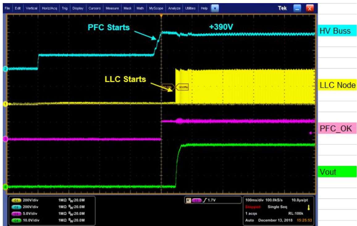
Figure 16 – Power up from 110 Vac
