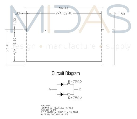
LED backlight brightness can be improved by changing the resistors on RA/RB, (the 750R resistors fitted as standard achieve a luminance of 150 cd/m2).
