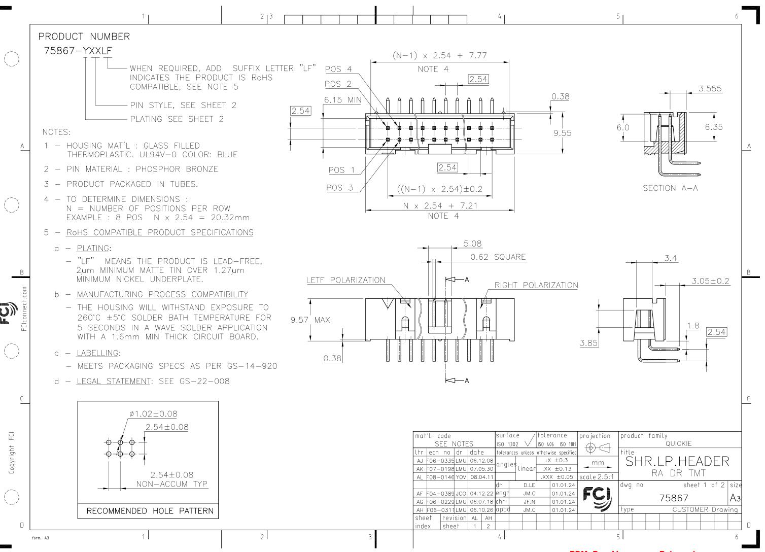
CORE RANGE Nbr OF LEFT PIN **RIGHT** POSITIONS | POLARIZATION | POLARIZATION STYLE NO NO 30  $2 \times 2$ 31  $2 \times 3$ NO NO 32 NO NO  $2 \times 4$ NO YES 01  $2 \times 5$ 02 2 x 7 NO YES YES YES 03 2 x 8 YES YES 04 2 x 10 YES YES 05 2 x 13 YES YES 33 2 x 15 YES YES 06  $2 \times 17$ YES YES 07  $2 \times 20$ 80  $2 \times 25$ YES YES 09  $2 \times 30$ YES YES  $2 \times 32$ YES YES 10
