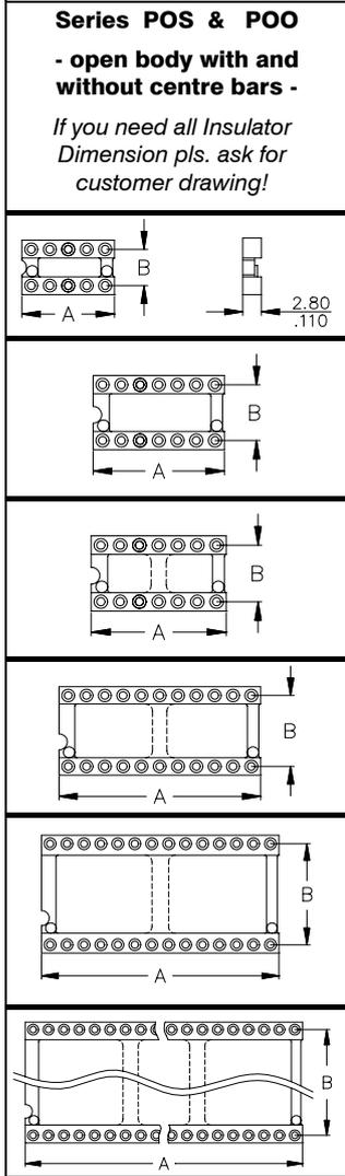
**POS sockets in 7,62mm/.300" DIP spacing are either supplied with or without bars in the centre depending on plastic wafer availability. If you need sockets without centre bars, then please always order with POO instead of POS.**
