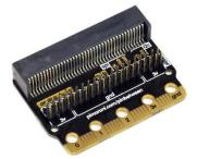
Pinbetween gives you access to all of the micro:bit's pins at the same time as using an edge-connector add-on, and it's completely solderless!
