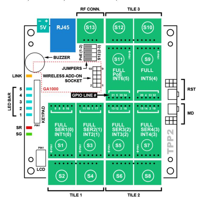
The TPP2 board features 6 x "M" and (6+1) x "C" sockets.
