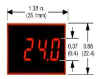
METER DEPTH: 1.00 in. (25.4mm)
