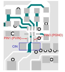
Figure 6: Two ends of Input decoupling Capacitor close to Pin 1 and Pin 3
