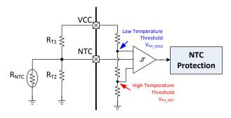
**Figure 5: NTC Protection Circuit**
