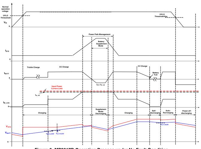
Figure 6: MP2617B Operation Process under No Fault Condition
