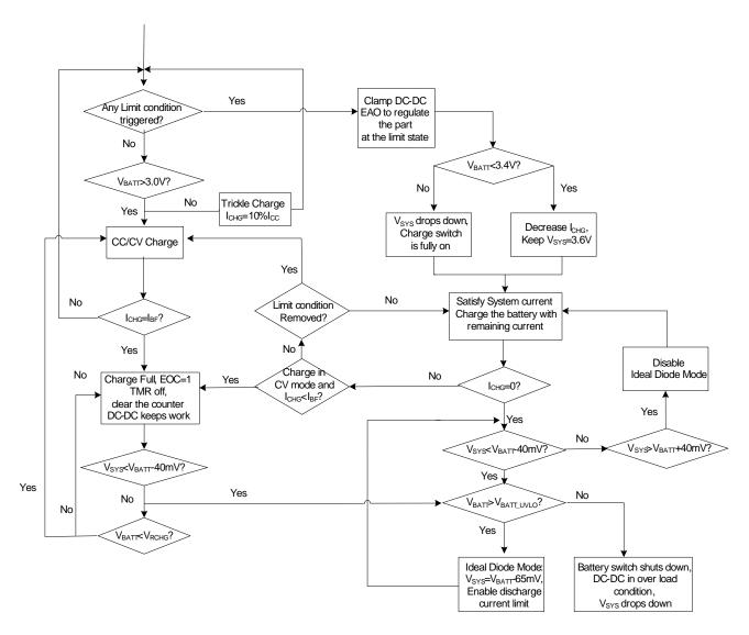
Figure 5: MP2617B Operation Flow Chart under No Fault Condition
