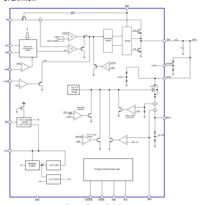
Figure 1—Function Block Diagram
