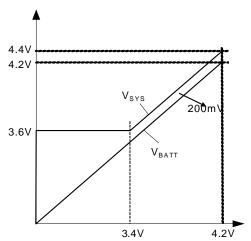
Figure 2 — MP2617B SYS Regulation Output
