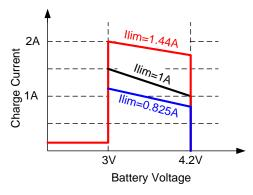
Figure 3:I<sub>CHG</sub> Variation with Different Input Current Limit
