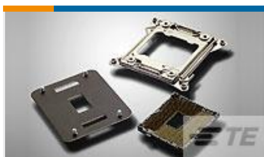
TE Part #1554653-1 SOCKET ASSY LGA2011, 0.38Au
