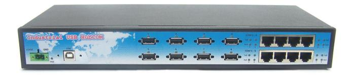
The HubCOM-880i-RM provides a lockable terminal power connector to supply 5V, 3A power to external device.
