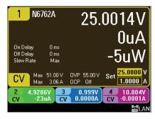
Figure 4. In Meter View, you can also view an enlarged view of one channel, displaying many settings and measured values, for that channel. A summary is shown for the other three channels.
