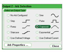
Figure 8. The Arb Selection menu is used to select which pre-programmed waveform will be applied to the output of the DC Power Module. Each of the four outputs can have a different waveform applied.
