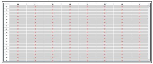
When the user hovers the mouse cursor over the GUI memory array, a pop-up appears to show the data in *HEX*, data in *ASCII*, *Address*, *Zone:* # and Zone Protection state (*Is locked*:) of that particular memory cell. This is illustrated in Figure 3-12.
