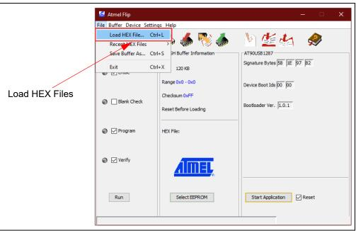
5. Proceed to load the  $I^2C$  firmware by navigating to the firmware found at: C:\Program Files (x86)\Microchip\Serial Memory Evaluation Kits\ $I^2C$ \Firmware
