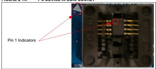
Once a device is installed in the SOIC socket, the user can then plug the USB Base Board into one of their computer's USB ports. Once the USB Base Board enumerates on the user's PC, open the GUI by selecting either the desktop icon (I<sup>2</sup>C GUI) or navigating to the Start Menu folder that was created when the DM160237 I<sup>2</sup>C Evaluation Kit GUI software was installed.
