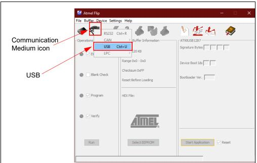
4. Once the communication between the PC and the AT90USB1287 (USB Base Board microcontroller) has been established, navigate to File and select "Load HEX Files" as shown in Figure 4-7.
