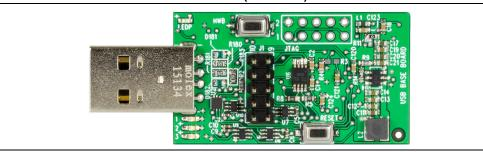
The I<sup>2</sup>C Socket Board also includes mikroBUS™ headers that allow the user to further develop applications by using the Socket Board with Microchip's extensive Development Tool offering. The Vcc for the mikroBUS™ operation can be selected by the user by changing jumper on header J3 to select either 3.3V or 5.0V.
