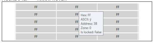
The user can change the content of a cell by double clicking a word address or memory cell in the GUI memory array. In order to change the content of a cell, the user should update the value, followed by pressing the **Update Cell** button. Once the cell is updated, the cell font will become *yellow*. This indicates to the user that they must program the device using the Program Feature (see **Section 3.11.5 "PROGRAM"** for additional information).
