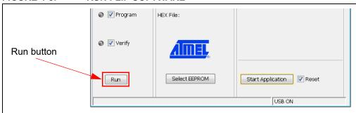
7. If the "Verified Pass" is reported in the FLIP Software Utility (see Figure 4-9), close the FLIP Software Utility and remove the USB Base Board from the PC. The USB Base Board Firmware Update procedure is complete.
