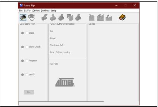
2. After opening the FLIP Software Utility, navigate to the Device Selection icon as shown below. Select the "AT90USB1287" as the device and press the **OK** button.
