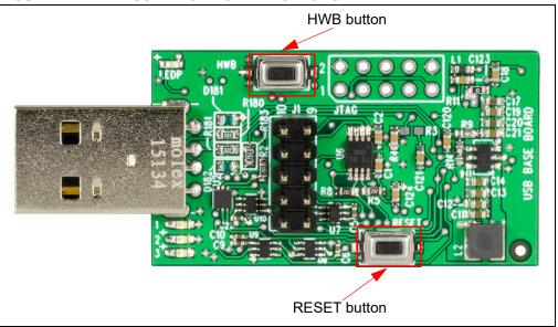
Once the **HWB** and **RESET** buttons have been located, use the specific press and hold sequence shown below to enable DFU mode on the USB Base Board:
